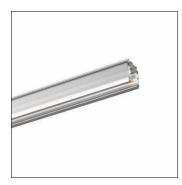
AX T, 3-phase track, installation type: suspended mounting, surface-mounted, mains connection: 220..240V/380..400V, AC, of extruded aluminium section, coated, grey, length: 3.000 mm, width: 32 mm, height: 33mm, protection rating (complete): IP20, insulation class (complete): insulation class I (protective earthing), certification: CE, ENEC, packaging unit: 1 piece
