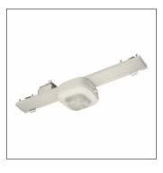
Licross®sensor PS2, slave, central control - connection to lighting or building management, dimmable, installation type: recessed, installation location: to the Licross® trunking rail, of sheet steel, protection rating (complete): IP20, insulation class (complete): insulation class I (protective earthing), certification: CE, UKCA, 1 x PIR movement sensor, 1 x light sensor, 1 x DALI, packaging unit: 1 piece
