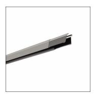
Licross®, trunking rail, of sheet steel, galvanised, coil coated, metallic grey (RAL 9006), length: 1.500 mm, width: 64 mm, height: 67mm, protection rating (complete): maximum IP64, depends on used inserts and accessories, insulation class (complete): insulation class I (protective earthing), certification: CE, UKCA, LABS conformity tested according to VDMA 24364:2018-05, packaging unit: 1 piece
