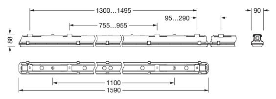
It is mandatory that the assembly instructions must be observed when planning and installing the electrical installation (to be found at www.siteco.de) Tolerances related to thermal, electrical and photometric data according to IEC 62722 Issued 22.12.2023 - Modifications and errors subject to change - Ensure that you always use the latest version -
