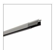
Licross®, trunking rail, of sheet steel, galvanised, coil coated, metallic grey (RAL 9006), length: 1.500 mm, width: 64 mm, height: 67mm, through-wiring: 7x 2.5mm², protection rating (complete): maximum IP64, depends on used inserts and accessories, insulation class (complete): insulation class I (protective earthing), certification: CE, UKCA, LABS conformity tested according to VDMA 24364:2018-05, packaging unit: 1 piece
