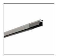
Licross®, trunking rail, of sheet steel, galvanised, coil coated, metallic grey (RAL 9006), length: 3.000 mm, width: 64 mm, height: 67mm, through-wiring: 7x 2.5mm², protection rating (complete): maximum IP64, depends on used inserts and accessories, insulation class (complete): insulation class I (protective earthing), certification: CE, UKCA, LABS conformity tested according to VDMA 24364:2018-05, packaging unit: 1 piece
