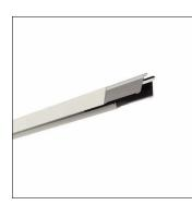
Licross<sup>®</sup>, trunking rail, of sheet steel, galvanised, coil coated, white, length: 3.000 mm, width: 64 mm, height: 67mm, through-wiring: 5x 2.5mm<sup>2</sup>, protection rating (complete): maximum IP64, depends on used inserts and accessories, insulation class (complete): insulation class I (protective earthing), certification: CE, UKCA, LABS conformity tested according to VDMA 24364:2018-05, packaging unit: 1 piece
