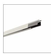
Licross<sup>®</sup>, trunking rail, of sheet steel, galvanised, coil coated, white, length: 3.000 mm, width: 64 mm, height: 67mm, protection rating (complete): maximum IP64, depends on used inserts and accessories, insulation class (complete): insulation class I (protective earthing), certification: CE, UKCA, LABS conformity tested according to VDMA 24364:2018-05, packaging unit: 1 piece
