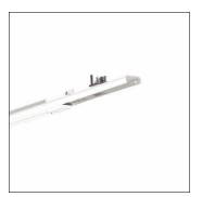
Modario®, track adapter insert, with plug, 5-pole, with phase selection, for trunking rail, 5 or 10-core, mains connection: 230/400V, track adapter insert, of sheet steel, coil coated, pure white, 2x system unit, max. weight load 5kg, length: 598mm, width: 48mm, protection rating (complete): for IP20 protection rating, insulation class (complete): insulation class I (protective earthing), certification: CE, packaging unit: 1 piece
