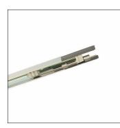
Modario<sup>®</sup> IP64, trunking rail, of sheet steel, galvanised, coated, pure white, 1length, length: 1.495 mm, width: 58 mm, height: 43mm, through-wiring: 5x 2.5mm<sup>2</sup>, with terminal, 5-pole, max. 2.5mm<sup>2</sup>, protection rating (complete): for IP64 protection rating, insulation class (complete): insulation class I (protective earthing), certification: CE, ENEC, VDE, standard: EN 60598, packaging unit: 1 piece
