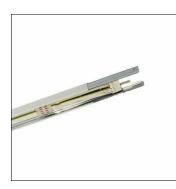
Modario<sup>®</sup>, trunking rail, of sheet steel, coated, pure white, 1-length, length: 1.495 mm, width: 58 mm, height: 43mm, through-wiring: 10x 2.5mm<sup>2</sup>, with terminal, 10-pole, max. 2.5mm<sup>2</sup>, protection rating (complete): for IP20/IP40 protection rating, insulation class (complete): insulation class I (protective earthing), certification: CE, ENEC, VDE, standard: EN 60598, packaging unit: 1 piece
