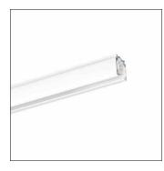
AX T, 3-phase track, installation type: suspended mounting, surface-mounted, mains connection: 220..240V/380..400V, AC, of extruded aluminium section, coated, white, length: 3.000 mm, width: 32 mm, height: 33mm, protection rating (complete): IP20, insulation class (complete): insulation class I (protective earthing), certification: CE, ENEC, packaging unit: 1 piece
