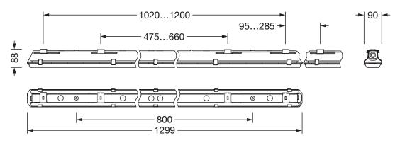
It is mandatory that the assembly instructions must be observed when planning and installing the electrical installation (to be found at www.siteco.de) Tolerances related to thermal, electrical and photometric data according to IEC 62722 Issued 10.11.2023 - Modifications and errors subject to change - Ensure that you always use the latest version -
