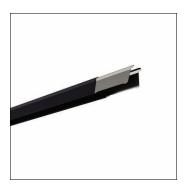
Licross®, trunking rail, of sheet steel, galvanised, coil coated, matt jet black (RAL 9005), length: 4.500 mm, width: 64 mm, height: 67mm, through-wiring: 5x 2.5mm², protection rating (complete): maximum IP64, depends on used inserts and accessories, insulation class (complete): insulation class I (protective earthing), certification: CE, UKCA, LABS conformity tested according to VDMA 24364:2018-05, packaging unit: 1 piece
