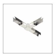
Licross® T-connector, white; trunking rail element of steel, galvanised, coated, with cable entry for six cables,  $\emptyset$  8.5..13mm; blank cover of PC/ABS, white, 3x connector of steel, galvanised, dimension: (LxWxH) = 300 x 197 x 67mm; for IP20/IP40 protection rating; certification: CE, UKCA; packaging unit: 1 piece
