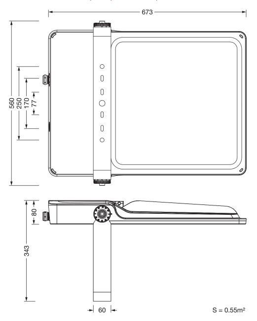
It is mandatory that the assembly instructions must be observed when planning and installing the electrical installation (to be found at www.siteco.de) Tolerances related to thermal, electrical and photometric data according to IEC 62722 Issued 24.02.2023 - Modifications and errors subject to change - Ensure that you always use the latest version -
