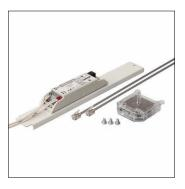
Monsun® 11/21sensor kit HC1, slave, local control, central control, dimmable, installation type: recessed, installation location: in the luminaire housing, of plastic, protection rating (complete): IP66, certification: CE, voltage type: AC, 1 x HF movement sensor, 1 x light sensor, 1 x DALI-2, 1 x status LED, packaging unit: 1 piece
