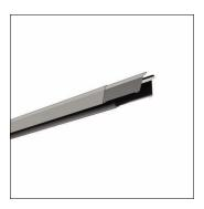
Licross®, trunking rail, of sheet steel, galvanised, coil coated, metallic grey (RAL 9006), length: 1.500 mm, width: 64 mm, height: 67mm, through-wiring: 9x 2.5mm², protection rating (complete): maximum IP64, depends on used inserts and accessories, insulation class (complete): insulation class I (protective earthing), certification: CE, UKCA, LABS conformity tested according to VDMA 24364:2018-05, packaging unit: 1 piece
