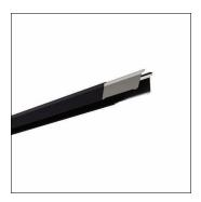
Licross®, trunking rail, of sheet steel, galvanised, coil coated, matt jet black (RAL 9005), length: 4.500 mm, width: 64 mm, height: 67mm, through-wiring: 9x 2.5mm², protection rating (complete): maximum IP64, depends on used inserts and accessories, insulation class (complete): insulation class I (protective earthing), certification: CE, UKCA, LABS conformity tested according to VDMA 24364:2018-05, packaging unit: 1 piece
