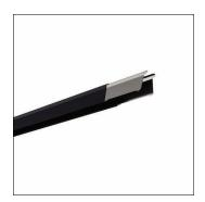
Licross®, trunking rail, of sheet steel, galvanised, coil coated, matt jet black (RAL 9005), length: 3.000 mm, width: 64 mm, height: 67mm, through-wiring: 5x 2.5mm², protection rating (complete): maximum IP64, depends on used inserts and accessories, insulation class (complete): insulation class I (protective earthing), certification: CE, UKCA, LABS conformity tested according to VDMA 24364:2018-05, packaging unit: 1 piece
