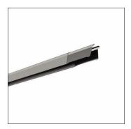
Licross®, trunking rail, of sheet steel, galvanised, coil coated, metallic grey (RAL 9006), length: 1.500 mm, width: 64 mm, height: 67mm, through-wiring: 5x 2.5mm², protection rating (complete): maximum IP64, depends on used inserts and accessories, insulation class (complete): insulation class I (protective earthing), certification: CE, UKCA, LABS conformity tested according to VDMA 24364:2018-05, packaging unit: 1 piece
