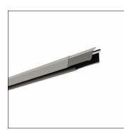
Licross<sup>®</sup>, trunking rail, of sheet steel, galvanised, coil coated, metallic grey (RAL 9006), length: 3.000 mm, width: 64 mm, height: 67mm, through-wiring: 5x 2.5mm<sup>2</sup>, protection rating (complete): maximum IP64, depends on used inserts and accessories, insulation class (complete): insulation class I (protective earthing), certification: CE, UKCA, LABS conformity tested according to VDMA 24364:2018-05, packaging unit: 1 piece
