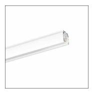
AX T, 3-phase track, installation type: suspended mounting, surface-mounted, mains connection: 220..240V/380..400V, AC, of extruded aluminium section, coated, white, length: 2.000 mm, width: 32 mm, height: 33mm, protection rating (complete): IP20, insulation class (complete): insulation class I (protective earthing), certification: CE, ENEC, packaging unit: 1 piece
