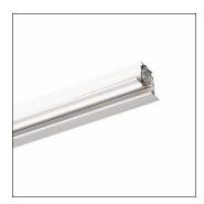
AX T, 3-phase track, installation type: recessed, mains connection: 220..240V/380..400V, AC, of extruded aluminium section, coated, white, length: 3.000 mm, width: 32 mm, height: 33mm, protection rating (complete): IP20, insulation class (complete): insulation class I (protective earthing), certification: CE, ENEC, packaging unit: 1 piece
