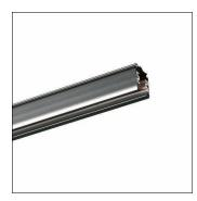
AX T, 3-phase track, installation type: suspended mounting, surface-mounted, mains connection: 220..240V/380..400V, AC, of extruded aluminium section, coated, jet black (RAL 9005), length: 1.000 mm, width: 32 mm, height: 33mm, protection rating (complete): IP20, insulation class (complete): insulation class I (protective earthing), certification: CE, ENEC, packaging unit: 1 piece
