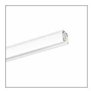
AX T, 3-phase track, installation type: suspended mounting, surface-mounted, mains connection: 220..240V/380..400V, AC, of extruded aluminium section, coated, white, length: 1.000 mm, width: 32 mm, height: 33mm, protection rating (complete): IP20, insulation class (complete): insulation class I (protective earthing), certification: CE, ENEC, packaging unit: 1 piece
