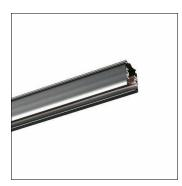
AX T, 3-phase track, installation type: suspended mounting, surface-mounted, mains connection: 220..240V/380..400V, AC, of extruded aluminium section, coated, jet black (RAL 9005), length: 3.000 mm, width: 32 mm, height: 33mm, protection rating (complete): IP20, insulation class (complete): insulation class I (protective earthing), certification: CE, ENEC, packaging unit: 1 piece
