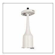
electrics components group, for Module 540 iQ, gear tray, control gear: ECG iQ, LED luminous flux: 1.590 lm, colour temperature: 2200K, with terminal, 6-pole, max. 2.5mm², mains connection: 230..240V, AC, 50/60Hz, start of lifetime: 13 W, end of service life: 13 W, reduction: 6 W, primary light characteristic: strongly asymmetric, width: 190 mm, height: 514mm, insulation class (complete): insulation class II (safety insulation), certification: CE, ENEC, VDE
