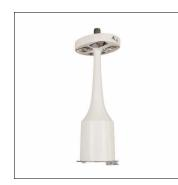
electrics components group, for Module 540 iQ, gear tray, control gear: ECG iQ, LED luminous flux: 3.110 lm, colour temperature: 4000K, with terminal, 6-pole, max. 2.5mm<sup>2</sup>, mains connection: 230..240V, AC, 50/60Hz, start of lifetime: 19 W, end of service life: 19 W, reduction: 9 W, primary light characteristic: symmetric, width: 190 mm, height: 514mm, insulation class (complete): insulation class II (safety insulation), certification: CE, ENEC, VDE
