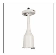
electrics components group, for Module 540 iQ, gear tray, control gear: ECG iQ, LED luminous flux: 1.590 lm, colour temperature: 3000K, with terminal, 6-pole, max. 2.5mm², mains connection: 230..240V, AC, 50/60Hz, start of lifetime: 11 W, end of service life: 11 W, reduction: 5 W, primary light characteristic: strongly asymmetric, width: 190 mm, height: 514mm, insulation class (complete): insulation class II (safety insulation), certification: CE, ENEC, VDF
