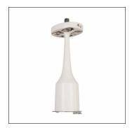
electrics components group, for Module 540 iQ, gear tray, control gear: ECG iQ, LED luminous flux: 3.110 lm, colour temperature: 2700K, with terminal, 6-pole, max. 2.5mm², mains connection: 230..240V, AC, 50/60Hz, start of lifetime: 24 W, end of service life: 26 W, reduction: 11 W, primary light characteristic: symmetric, width: 190 mm, height: 514mm, insulation class (complete): insulation class II (safety insulation), certification: CE, ENEC, VDE
