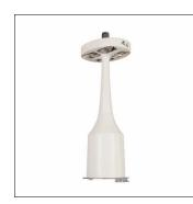
electrics components group, for Module 540 iQ, gear tray, control gear: ECG iQ, LED luminous flux: 4.100 lm, colour temperature: 2700K, with terminal, 6-pole, max. 2.5mm<sup>2</sup>, mains connection: 230..240V, AC, 50/60Hz, start of lifetime: 34 W, end of service life: 36 W, reduction: 15 W, primary light characteristic: asymmetric, width: 190 mm, height: 514mm, insulation class (complete): insulation class II (safety insulation), certification: CE, ENEC, VDE
