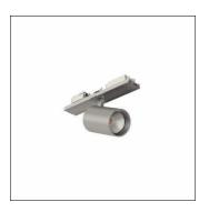
Licross® Spot 31, directional spotlight, light control with lens, of plastic, LED rated luminous flux: 3.680lm, light colour: 940, control gear: ECG, with plug, 3-pole, with phase selection, mains connection: 220..240V, AC, 50/60Hz, of aluminium, metallic grey (RAL 9006), length: 140mm, diameter: 90mm, protection rating (complete): IP20, insulation class (complete): insulation class I (protective earthing), certification: CE, packaging unit: 1 piece
