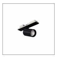
Licross® Spot 31, directional spotlight, light control with lens, of plastic, LED rated luminous flux: 3.680lm, light colour: 940, control gear: ECG DALI, with plug, 5-pole, mains connection: 220..240V, AC, 50/60Hz, of aluminium, jet black (RAL 9005), length: 140mm, diameter: 90mm, protection rating (complete): IP20, insulation class (complete): insulation class I (protective earthing), certification: CE, packaging unit: 1 piece
