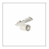
Licross® Spot 31, directional spotlight, light control with lens, of plastic, LED rated luminous flux: 3.720lm, light colour: 940, with plug, 3-pole, with phase selection, mains connection: 220..240V, AC, 50/60Hz, of aluminium, traffic white (RAL 9016), length: 140mm, diameter: 90mm, protection rating (complete): IP20, insulation class (complete): insulation class I (protective earthing), certification: CE, packaging unit: 1 piece
