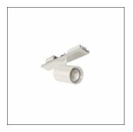
Licross® Spot 31, directional spotlight, light control with lens, of plastic, LED rated luminous flux: 5.250lm, light colour: 940, with plug, 5-pole, mains connection: 220..240V, AC, 50/60Hz, of aluminium, traffic white (RAL 9016), length: 140mm, diameter: 90mm, protection rating (complete): IP20, insulation class (complete): insulation class I (protective earthing), certification: CE, packaging unit: 1 piece
