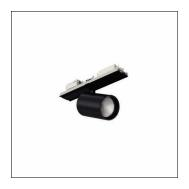
Licross® Spot 31, directional spotlight, light control with lens, of plastic, LED rated luminous flux: 5.190lm, light colour: 940, control gear: ECG DALI, with plug, 5-pole, mains connection: 220..240V, AC, 50/60Hz, of aluminium, jet black (RAL 9005), length: 140mm, diameter: 90mm, protection rating (complete): IP20, insulation class (complete): insulation class I (protective earthing), certification: CE, packaging unit: 1 piece
