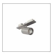
Licross® Spot 31, directional spotlight, light control with lens, of plastic, LED rated luminous flux: 5.250lm, light colour: 940, control gear: ECG, with plug, 3-pole, with phase selection, mains connection: 220..240V, AC, 50/60Hz, of aluminium, metallic grey (RAL 9006), length: 140mm, diameter: 90mm, protection rating (complete): IP20, insulation class (complete): insulation class I (protective earthing), certification: CE, packaging unit: 1 piece
