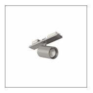
Licross® Spot 31, directional spotlight, light control with lens, of plastic, LED rated luminous flux: 5.190lm, light colour: 940, control gear: ECG DALI, with plug, 5-pole, mains connection: 220..240V, AC, 50/60Hz, of aluminium, metallic grey (RAL 9006), length: 140mm, diameter: 90mm, protection rating (complete): IP20, insulation class (complete): insulation class I (protective earthing), certification: CE, packaging unit: 1 piece
