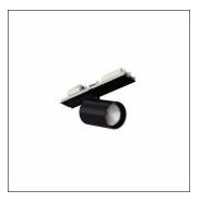
Licross® Spot 31, directional spotlight, light control with lens, of plastic, LED rated luminous flux: 5.140lm, light colour: 940, control gear: ECG DALI, with plug, 5-pole, mains connection: 220..240V, AC, 50/60Hz, of aluminium, jet black (RAL 9005), length: 140mm, diameter: 90mm, protection rating (complete): IP20, insulation class (complete): insulation class I (protective earthing), certification: CE, packaging unit: 1 piece
