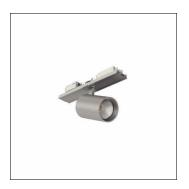
Licross® Spot 31, directional spotlight, light control with lens, of plastic, LED rated luminous flux: 5.190lm, light colour: 940, control gear: ECG, with plug, 3-pole, with phase selection, mains connection: 220..240V, AC, 50/60Hz, of aluminium, metallic grey (RAL 9006), length: 140mm, diameter: 90mm, protection rating (complete): IP20, insulation class (complete): insulation class I (protective earthing), certification: CE, packaging unit: 1 piece
