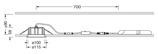
It is mandatory that the assembly instructions must be observed when planning and installing the electrical installation (to be found at www.siteco.de) Tolerances related to thermal, electrical and photometric data according to IEC 62722 Issued 30.03.2024 - Modifications and errors subject to change - Ensure that you always use the latest version -
