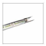
Modario®, trunking rail, of sheet steel, coated, pure white, 10x system unit 299mm 10-core and 2x system unit 1495mm 2-core, length: 2.990 mm, width: 58 mm, height: 43mm, through-wiring: 12x 2.5mm², with terminal, 10+2-pole, max. 2.5mm², protection rating (complete): for IP20/IP40 protection rating, insulation class (complete): insulation class I (protective earthing), certification: CE, ENEC, VDE, standard: EN 60598, packaging unit: 1 piece
