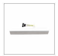
Modario® 31 feed-out, white; wiring connection compartment of sheet steel, galvanised, coated, with cable entry for four cables, Ø 8.5..13mm; 1x blank cover of PC/ABS, white; connection via terminal, 10-pole, max. 2.5mm², internal wiring halogen-free; dimension: (LxWxH) = 449 x 58 x 43mm; IP40; insulation class: insulation class I (protective earthing); certification: CE, UKCA; packaging unit: 1 piece
