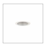
Lunis 31, -L, downlight, light control with reflector, light emission: direct distribution, LED rated luminous flux: 1.700lm, light colour: 840, mains connection: 220..240V, AC/DC, 0/50..60Hz, housing, of aluminium, white, protection rating (complete): IP20, protection rating (on room side): IP54, insulation class (complete): insulation class II (safety insulation), certification: CE, ENEC, packaging unit: 1 piece
