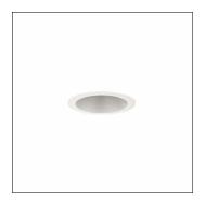
Lunis 31, -L, downlight, light control with reflector, light emission: direct distribution, LED rated luminous flux: 1.600lm, light colour: 840, mains connection: 220..240V, AC/DC, 0/50..60Hz, housing, of aluminium, white, protection rating (complete): IP20, protection rating (on room side): IP54, insulation class (complete): insulation class II (safety insulation), certification: CE, ENEC, packaging unit: 1 piece
