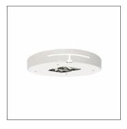
electrics components group, for Large Bell iQ, luminous flux: 5.180 lm, colour temperature: 3000K, mains connection: 230..240V, AC, 50/60Hz, start of lifetime: 34 W, end of service life: 38 W, reduction: 16 W, primary light characteristic: asymmetric, gear tray, insulation class (complete): insulation class II (safety insulation), certification: CE, ENEC, VDE
