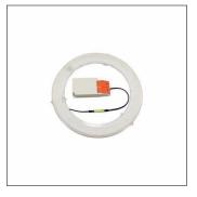
Lunis R, luminaire insert, rated luminous flux: 4.100lm, light colour: 830, control gear: ON/OFF Multilumen, mains connection: 220..240V, AC, 50/60Hz, rated input power: 25.9W, primary light control with lens, of plastic, primary optical cover: cover, of PMMA, light emission: direct distribution, protection rating (complete): IP20, certification: CE, packaging unit: 1 piece
