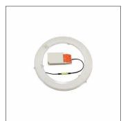
Lunis R, luminaire insert, rated luminous flux: 4.400lm, light colour: 830, control gear: DALI 2, mains connection: 220..240V, AC, 50/60Hz, rated input power: 27W, primary light control with lens, of plastic, primary optical cover: cover, of PMMA, light emission: direct distribution, protection rating (complete): IP20, certification: CE, packaging unit: 1 piece
