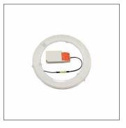
Lunis R, luminaire insert, rated luminous flux: 4.400lm, light colour: 840, control gear: DALI 2, mains connection: 220..240V, AC, 50/60Hz, rated input power: 25W, primary light control with lens, of plastic, primary optical cover: cover, of PMMA, light emission: direct distribution, protection rating (complete): IP20, certification: CE, packaging unit: 1 piece
